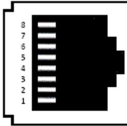
On the rear panel of 3110C, there have two RJ-45 connectors provides standard Ethernet connections for channel A (on upper side) and channel B (on below side).
