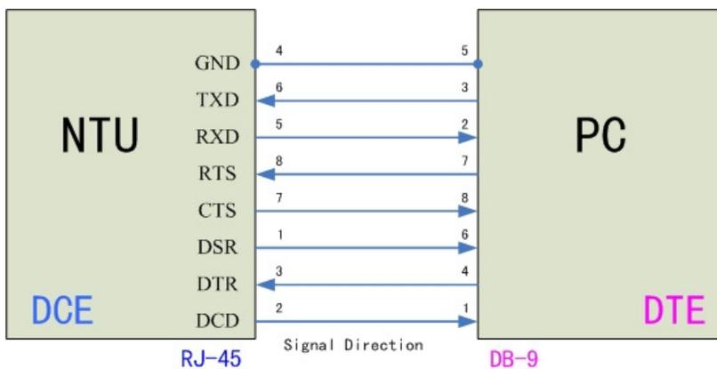
The pin assignment of RJ-45 modular jack on the console cable:
