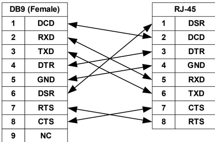
The signal direction of console cable:
