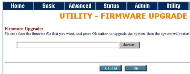
Select the firmware file name by click **Browse** on your PC or NB and press **OK** button to upgrade. The system will reboot automatically after finish the firmware upgrade operation.
