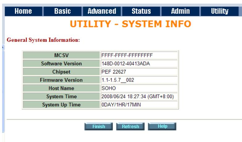
There will display general system information including: MCSV, software version, chipset, firmware version, Host Name, System Time and System Up Time.
