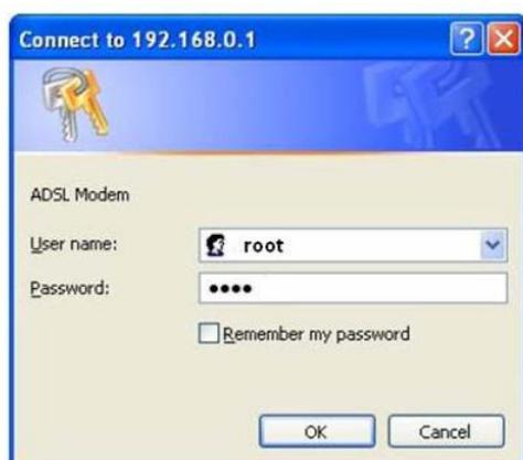
The factory default management IP and subnet mask are 192.168.0.1 and 255.255.255.0. If you haven't any user profile for line card before, enter the factory default user name "root" and password "root" to login the device.
