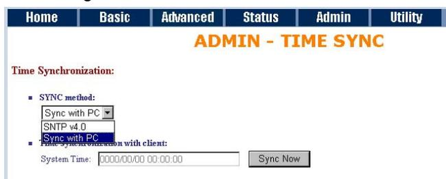
For using the SNTP, select **SNTP v4.0**.
