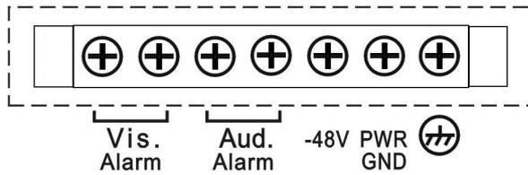
There are not using the alarm connectors (Vis. Alarm and Aud. Alarm) for ATM based line card.
